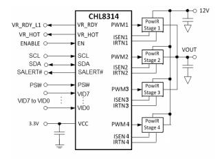
Figure 1: CHL8314 Basic Application Circuit
