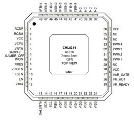
Figure 2: CHL8314 Package Top View
