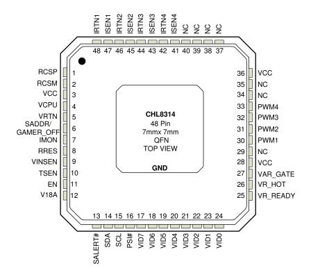
Figure 3: CHL8314 Top View Enlarged
